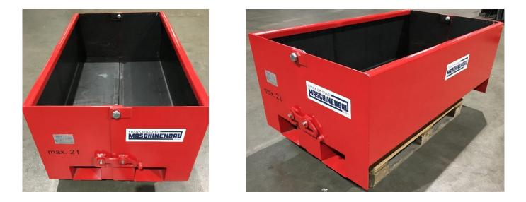
An additional manually swiveling bracket locks the scrap box so that the bottom of the scrap box cannot open during transport by the forklift.
